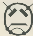
Fig. 254. The two diodes of Fig. 253 (a) may be combined in one envelope with a single cathode
