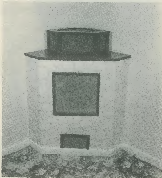
One of the two brick corner enclosures built into a new bungalow (see "High Fidelity Built In"). This incorporates a Wharfedale W15 bass unit, a Super 3 and Super 8 being fitted in the cabinet on top
