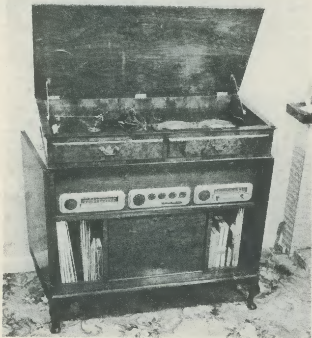
Installing high fidelity equipment without upsetting the harmony with other furniture. This "Queen Anne" cabinet houses two Quad power amplifiers as well as a Quad control unit and a.m. and f.m. tuners. Also visible are a Thorens TD124 turntable and a Tandberg Series 6 tape recorder
